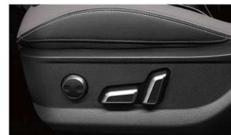
Driver's seat with 8-direction electric adjustable + memory + welcome functions
